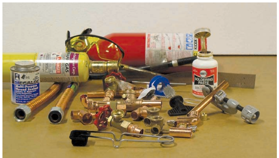
Some of the tools and parts you might need for soldering copper tubing include solder, flux, Teflon tape, and fittings.
