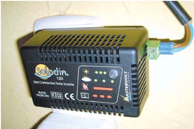
The Soladin 120 inverter plugged into the wall socket.
