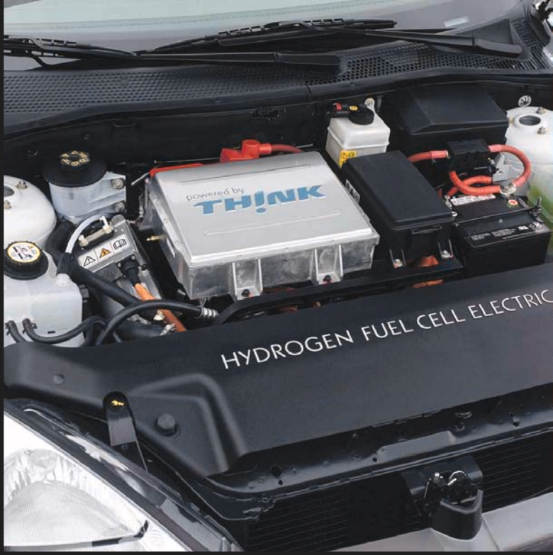
A fuel cell vehicle, like this Ford Focus, involves special packaging challenges.
